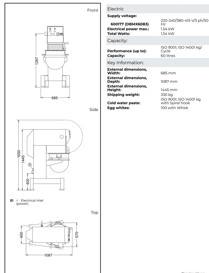
Planetary Mixers Planetary Mixer, 60 lt
