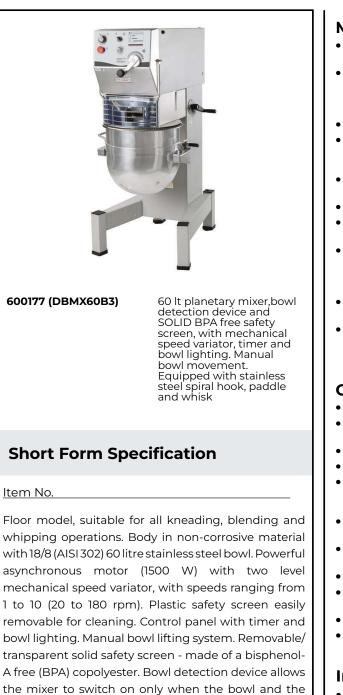
safety screen are properly installed and positioned together. Supplied with 3 tools: stainless steel spiral kneading
